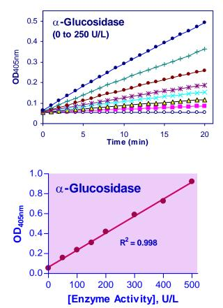
Kinetics of  $\alpha$ -glucosidase reaction in 96-well plate assay
