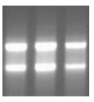
Fig. 7. Agarose gel image of human whole blood RNA isolated from 3 different donors.
